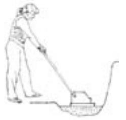
3. Fill the trench with 4 inches of well-graded gravel material, (1/2" minus or 3/4" minus road mulch) compacting firmly in 2-inch layers to ensure proper compaction. Note: Hand tamping tools may be used, but vibrating compaction equipment is recommended.
